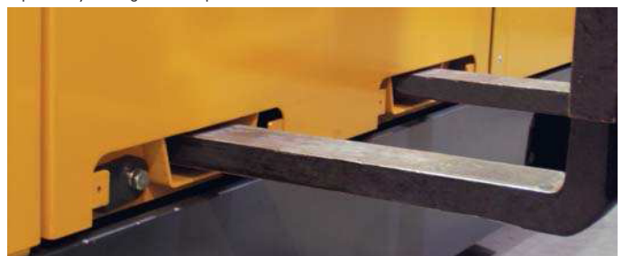
Rapid battery exchange with fork pockets
