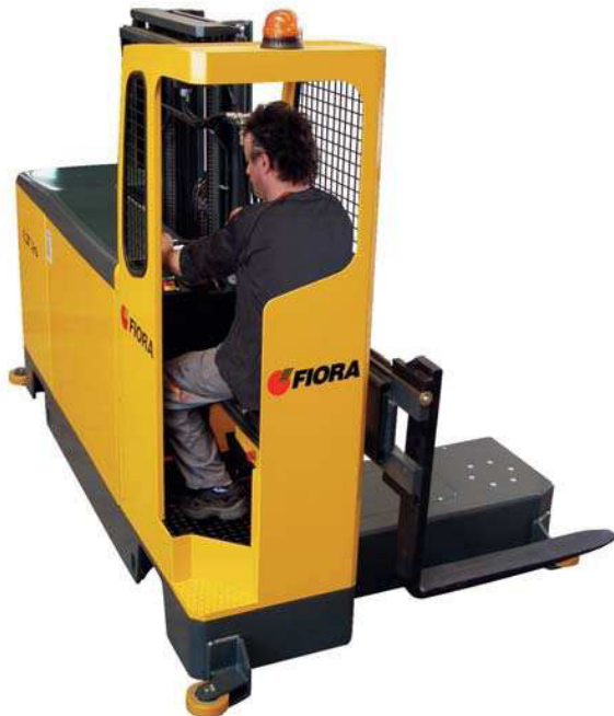
Ergonomic cabin with access on the corridor side
